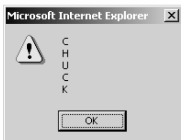
Figure 6-3. Each line displayed is a distinct argument handed to the createList() function.
